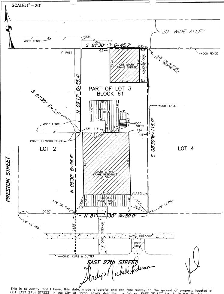
This is to certify that I have, this date, made a careful and accurate survey on the ground of property located at 604 EAST 27th STREET, in the City of Bryan, Texas, described as follows: PART OF LOT No. 3, BLOCK No. 61, of ORIGINAL TOWNSITE ADDITION, according to the plat recorded in Volume "H", Page 721, of the Deed Records of ORIGINAL TOWNSITE AD Brazos County, Texas.
